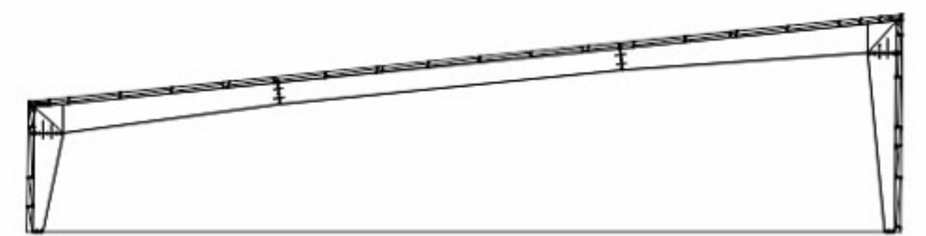
SINGLE SLOPE - RF (CLEAR SPAN)
