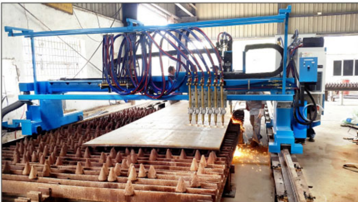
3.1 CNC Plasma Cutting: ■ Size: 4.0 m x 18.0 m.
