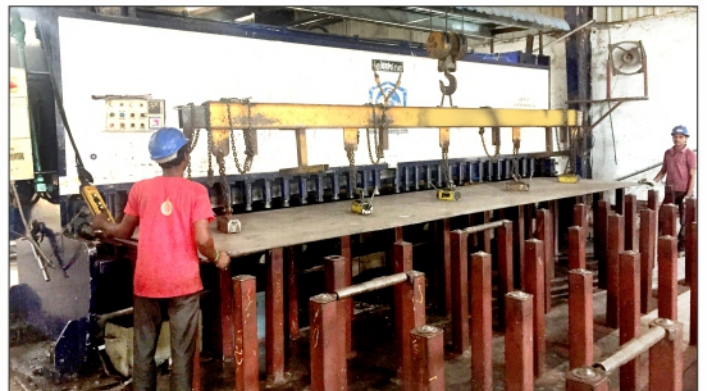
3.2 Shearing Machine: ■ Size: 6.3 m max cut length. ■ Thickness: 15.0 mm max.
