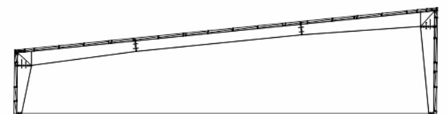
SINGLE SLOPE - RF (CLEAR SPAN)
